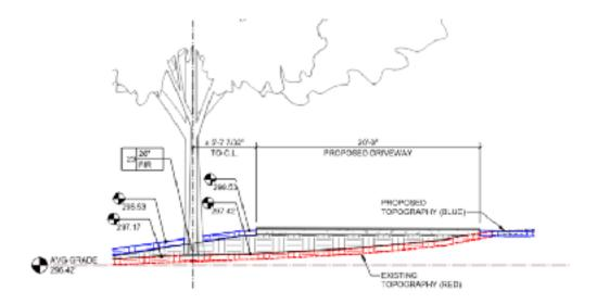
As it specifies, the red line is the existing topography, the blue line the proposed topography. Installation of the driveway will not require any ground disturbance within the drip line of the tree; it will rather require a slight amount of fill. Therefore, since no roots will be impacted, an advanced root assessment is not necessary.
